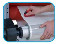
In order to protect the laminating rollers from unsafe operation when not using a proper cutter, a safety cutter is delivered with the machine. The quality of your lamination job and your investment are preserved for years.
