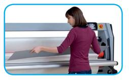
The machine is delivered with a metal feeding tray in order to reduce material waste and to save time when installing the film on the machine.
