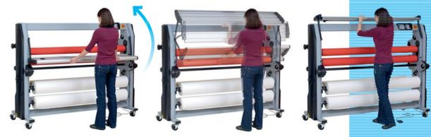
The feeding tray pivots upwards leaving a full and secure access to the machine when loading the film. In upper position, the driving motor is shut, preventing the operator from any injury during the operation.
